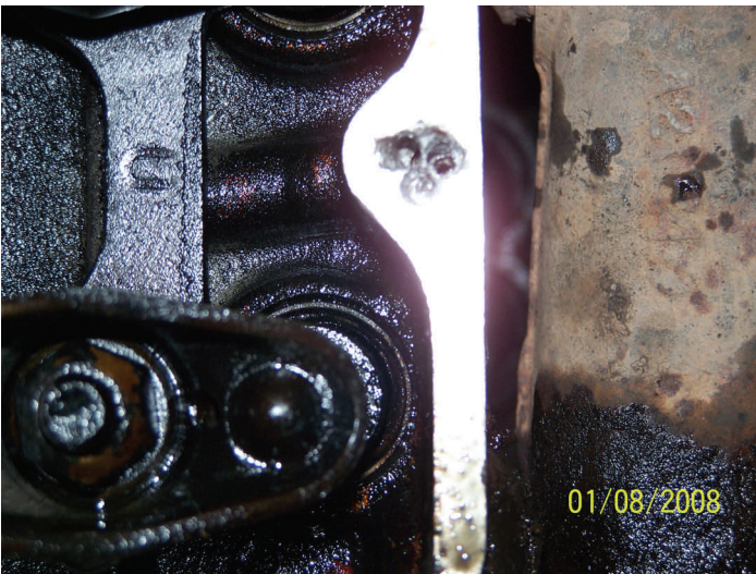
How NOT to repair a bad valve cover Bolt
